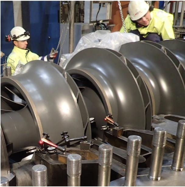
**Figure 1.** Compressor rotor axial alignment.
