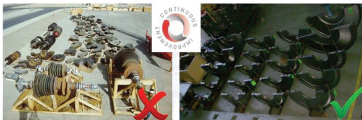
Figure 3. Productivity tools: racks for handling diaphragms.
